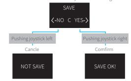
setting ,one tap setting button under setting window to save temporarily and go back to main screen, resets after
