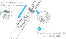
All screw holes on the remote can be used as a extension port, add any suitable accessories as needed.
