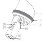
\*GoPro adapter [3] can be manually removed and install to thread hole[5]
