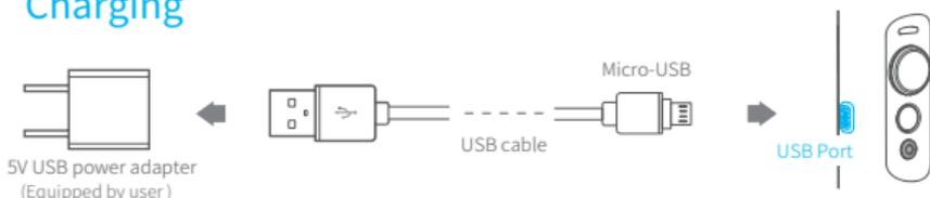
After power off, connect the USB cable to USB port, and connect with 5V USB power adapter (equipped by user) by USB cable .
