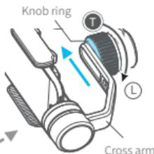
If the iPhone tilted to the left, then loose the knob ring, move the cross arm to the right, try to adjust to the best balance then tight it.
