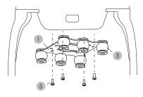
Install the damping ball to the Adapter(Down). 将减震球另一端按下图装入至云台下挂板中
