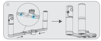
Installation and disassembly of a series gimbal: ①Install the a series gimbal, tighten the retaining ring;②Loosen the retaining ring and remove the a series gimbal gently.
